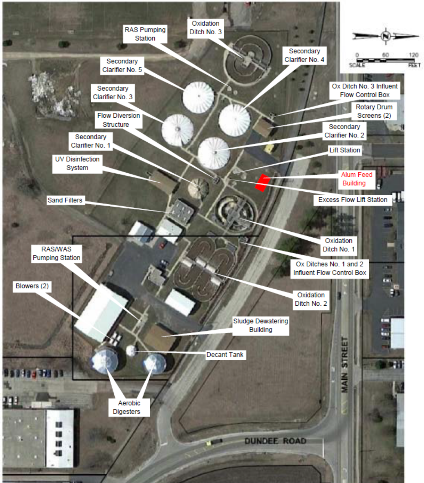
Exhibit 4-1: East WWTF Aerial View – Recommended Plan – 1.0 mg/L TP Limit Village of Huntley, IL
